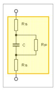
No exact data, but for the (dry) sponge slices I used (4 x 3 x 0.8 cm)rough estimates are:compresseduncompressedRs : 0.1k $5k\Omega$ Rp:  $50k \Omega$  $1M\Omega$ C: 100nF0.5nF
